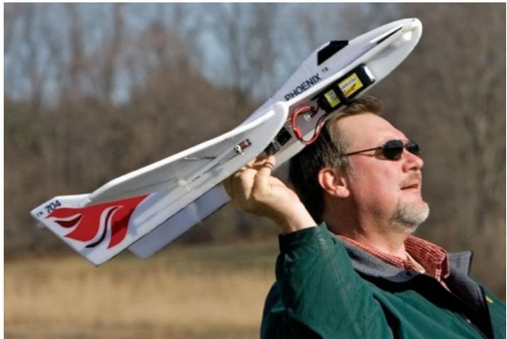
Another technique is to hold the model from above with you hand just forward of the balance point. You can then use an upward underhand motion to launch the plane.
