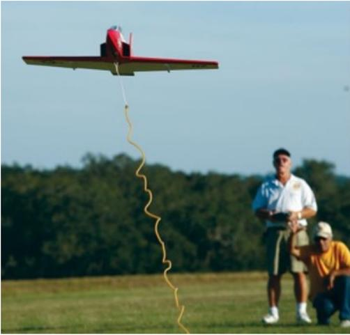
When it comes to smaller, electric powered ducted-fan jet models, a safe and easy way to launch is using a bungee assist. With a buddy taking care of the model release, you will have both your hands on the radio and you won't be distracted and can deal with the controls to keep the model flying straight and true until you get up on step and have enough airspeed for a safe climb out.
