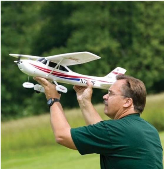
Holding the fuselage too far aft usually causes the model to pivot nose down during the launch. A far better and safer way is to have a friend hold the plane with two hands (one in front of the wing and one aft), so it can be launched sidewinder style, not exactly overhead.
