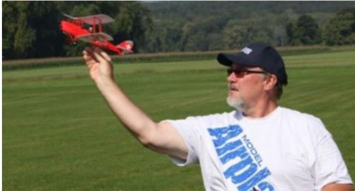
Remember to always launch your model while facing straight into the wind. Don't throw your model downwind (with wind at your back), this will cause the model to stall, lose lift possibly striking the ground.
